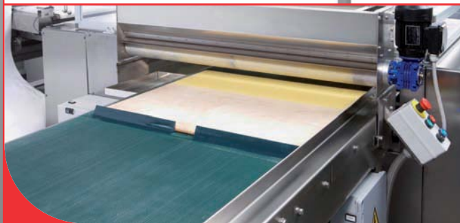
Reciprocating Belt Panner with a tray feeding cross conveyor, complete with a corn meal duster to dust the peelboards before panning.
